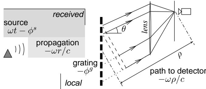
Fig. 1. Phase contributions in Fourier spectrometry
