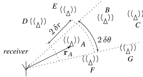
Fig. 7. Signal selection by direction and range
