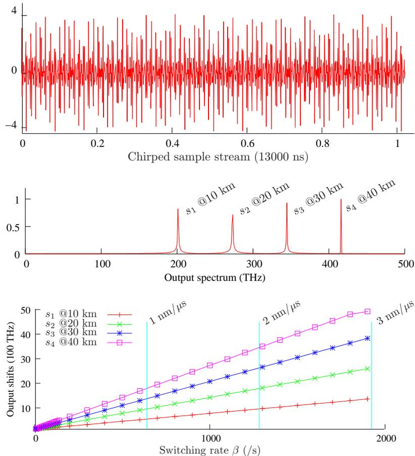
Fig. 8. Verification of the effect by chirped sampling
